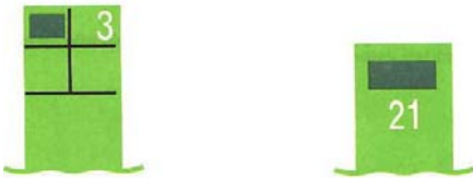
Figure 3-1. Lateral port marks.
