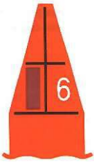
Figure 3-2. Lateral starboard marks.
